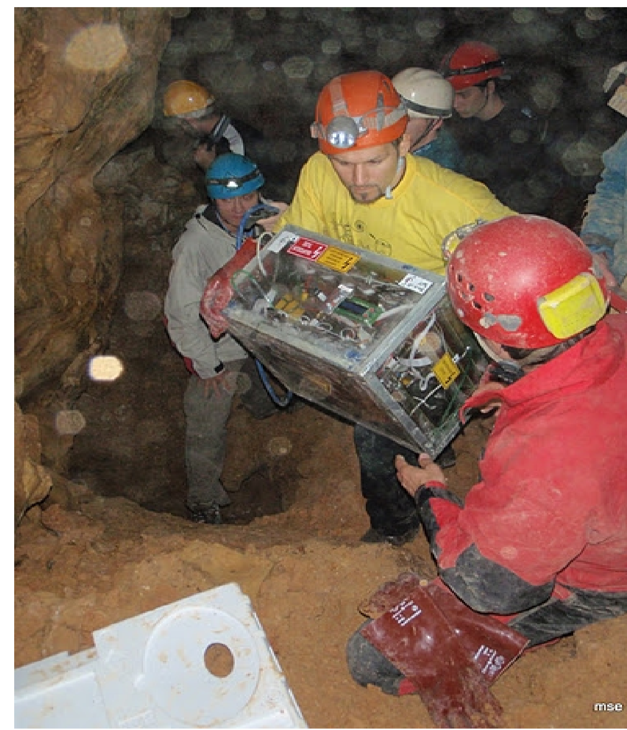
Fig. 2: The Close Cathode Chamber-based tracking device measures the cosmic background in a tunnel system in Felsenkeller Germany ( left panel ) and its installation in the Ariadne Cave System in Pilis Mountains, Hungary ( right panel ).
