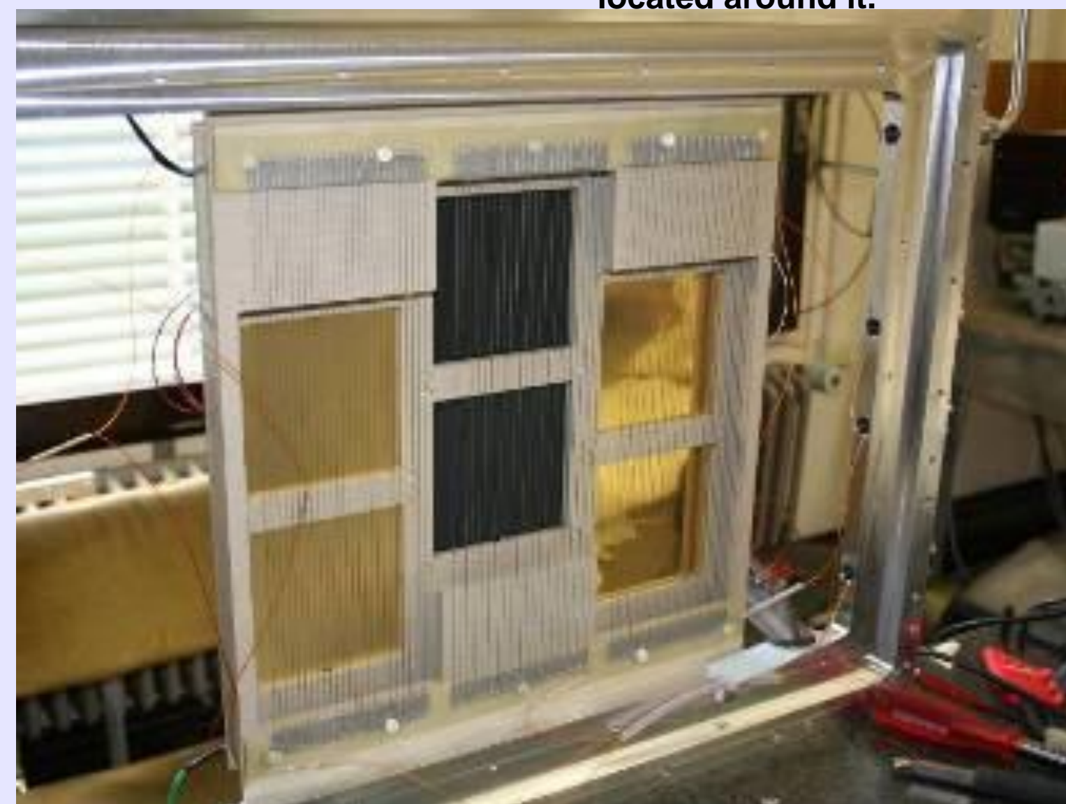
Figure 8.: Photosensitive GEM modules in the prototype (left) and its back side with the radiator (right) and the mirror (below)
