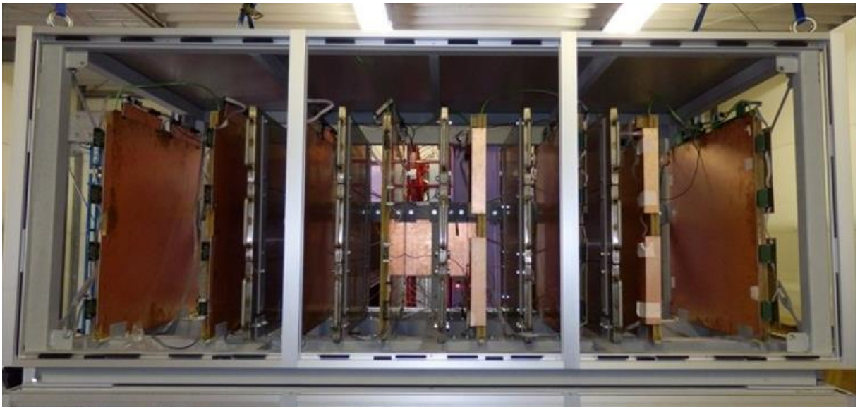
Figure 10. The first MWPC system which was installed in a strong steel framed box approximately 3 km from the crater. There are lead absorber walls between the detectors which improves the noise performance [17].
