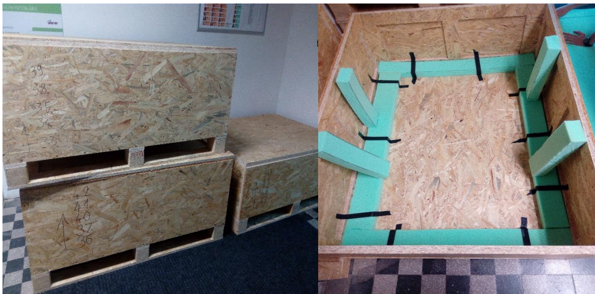
Figure 42. The transportation boxes for the detectors (left) and the sliced polymer foams inside the box with defined sizes, acting as spacers between the detectors (right).
