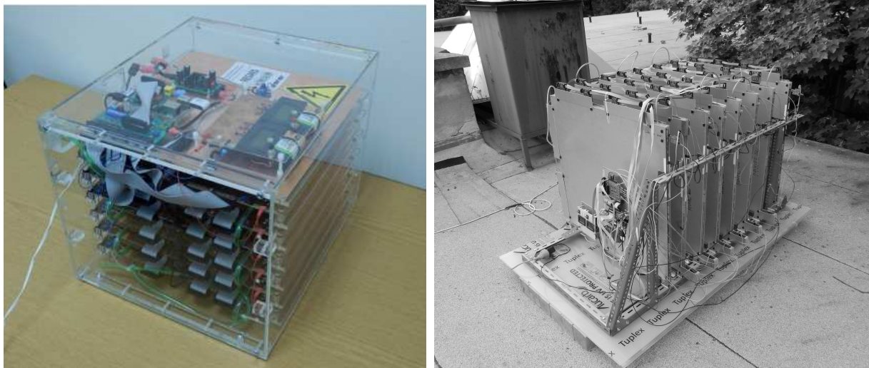
Figure 44: Photos about the developed tracking systems: a CCC-based tracker for underground muography ( left ) and a MWPC-based system ( right ) for imaging by tracking the near-horizontal muons.
